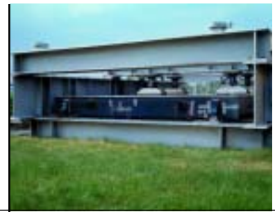
Automated axle-load simulator tests the scale's durability.
